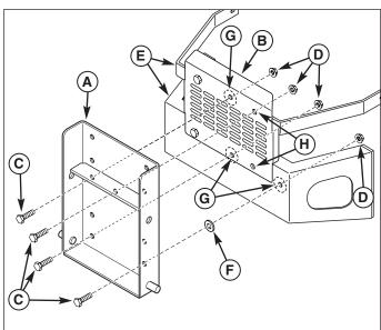
Figure 1. Install Hitch Plate (Flat Style Bumper)
